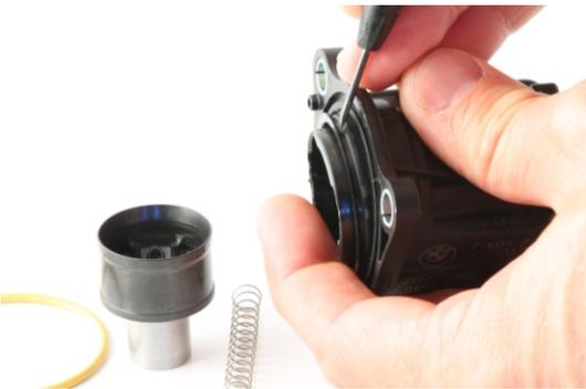
Note that this plastic piece can become brittle over time and damage may occur during removal. If it breaks, you'll still be able to continue with the DV+ installation as this part isn't used, but you won't be able to re-install the factory diverter again.
