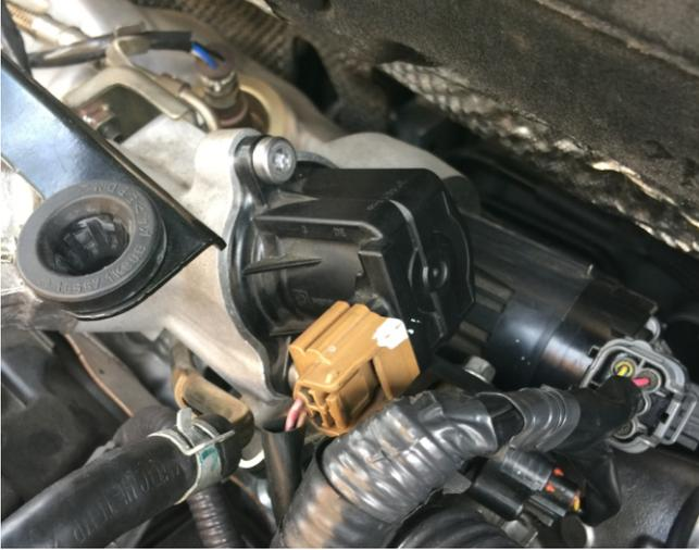
On Renault Clio RS engines, the factory diverter is mounted on a plastic housing joined by hoses. There is also a mounting bracket that holds the housing in place. It is easiest to first remove the screws holding this housing, which makes it easier to access the three screws that retain the factory diverter.
