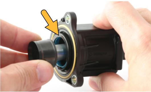
Pull the piston and spring out of the body, then remove the yellow o-ring. This will leave the plastic ring indicated by the arrow, which **MUST BE REMOVED** before the DV+ is installed. Lever it gently and work your way around.
